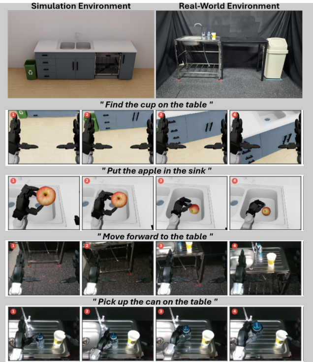
Fig. 4. Simulation and real-world environments and trajectories. Top left: simulated kitchen environment; top right: real-world environment. Rows 2–3: simulation locomotion/manipulation trajectory sequences from the dataset. Rows 4–5: real-world locomotion/manipulation trajectories.
